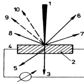
*Fig. 4 Signals in REM – 1 – primary electron beam, 2 – sample, Electrons: 3 – passing, 4 – absorbed, 5 – diffused, 6 – reflected, 7 – secondary, 8 – Auger's, 9 – characteristic RTG emission, 10 – continuous RTG emission*
