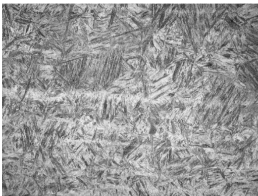
Fig. 6 Microstructure of ArmoX 500 – area of HAZ close to weld metal (mg. 500x )
