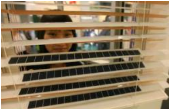
Fig. 7 Photovoltaic panels on window
