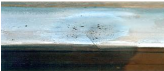
Fig.8 Squats - A typical crack formation in the shape V of a tread in the railhead
