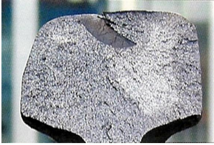
Fig.6 this shows the development of a crack
