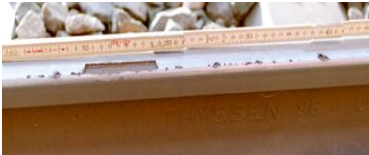
Fig. 10 example Shelling in the final stage
