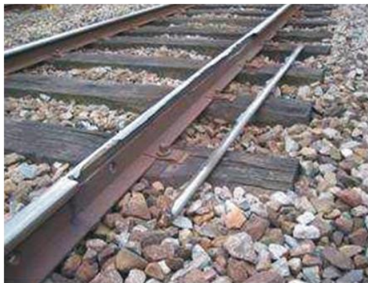
Cracking spreads in the direction of the length of the rail
