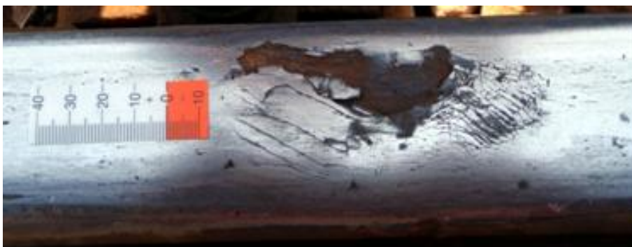
Fig. 9 example defect wheelburns
