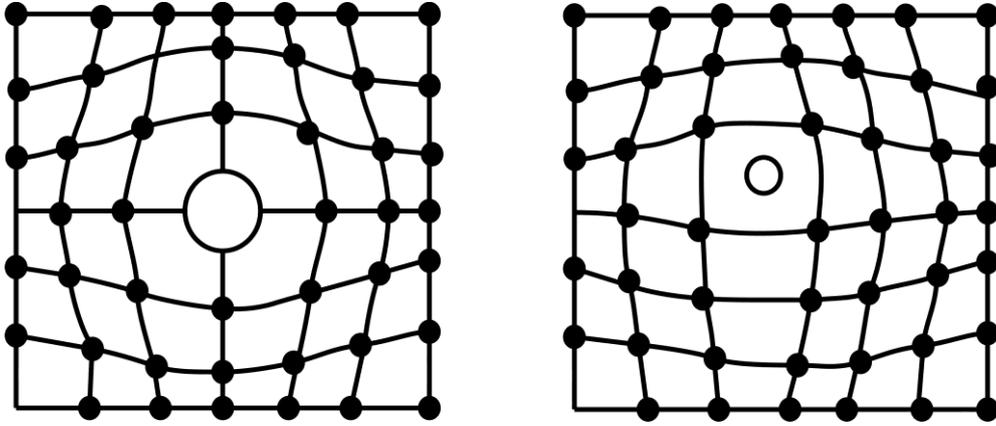
Fig. 2 Substitutional and interstitial impurity atoms.
