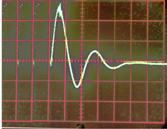
Fig. 1 Oscillogram of a pulse shape. Time-base sweep, 50  $\mu$ s/division.
