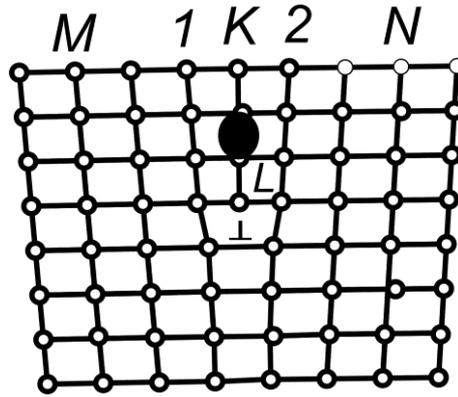
Fig. 4 Interaction between dislocation and impurity atom.
