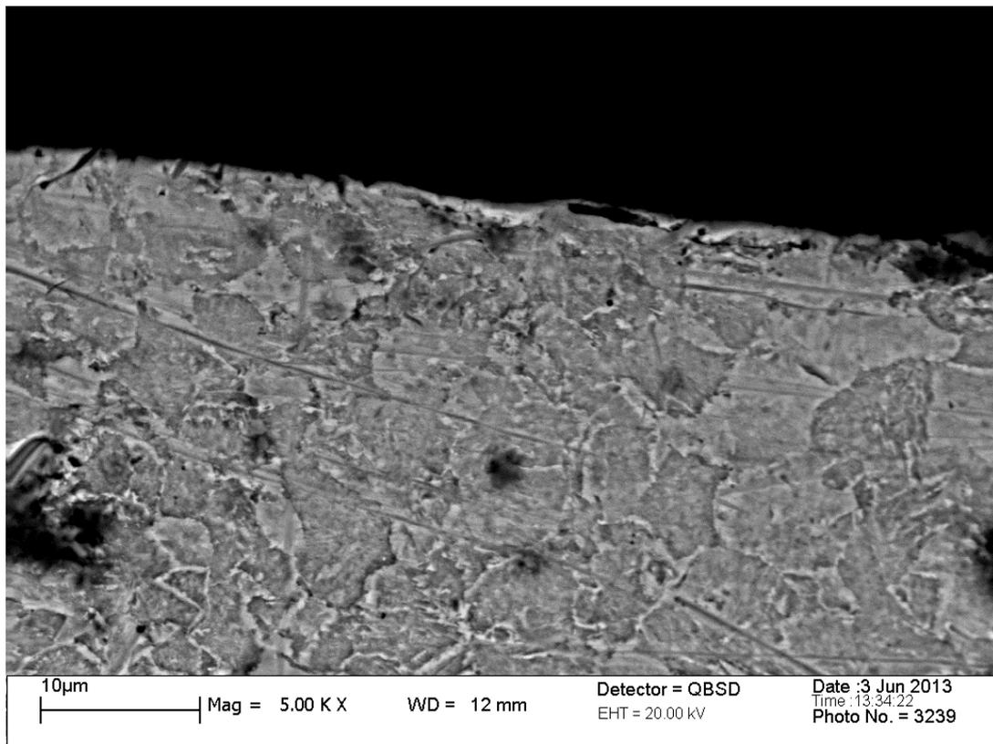
**Fig. 3** Formation of fine- grained structure on the surface of a sample made of Steel 45 during magnetic pulse hardening (2 pulses, 6 kJ)
