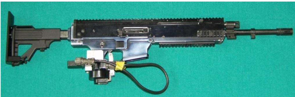
Fig. 9 MSBS-5,56 K-01 rifle prepared to the installation on the test stand
