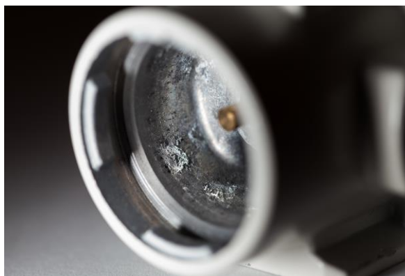
Fig. 2 Corrosion attack of casting AF 20
