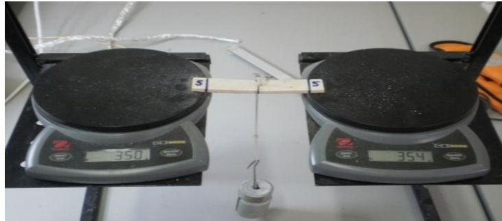
Fig. 2 Bending device (three point method) of the testing machine
