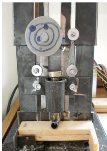
Fig. 6 Fatigue test of composite specimens
