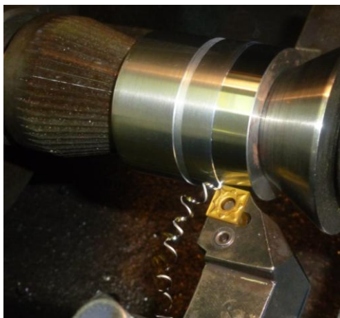
Fig. 5 Longitudinal surface turning of the testing sample no.1
