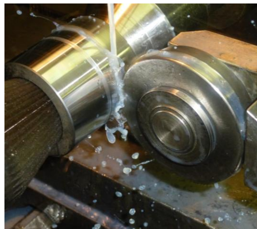
Fig. 6 Burnishing of rotational surface of the sample.1 with feed motion f_1 (experiment 1)
