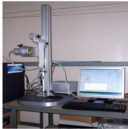
Fig. 3 Certification panel measuring accuracy device Tribotest [4]
