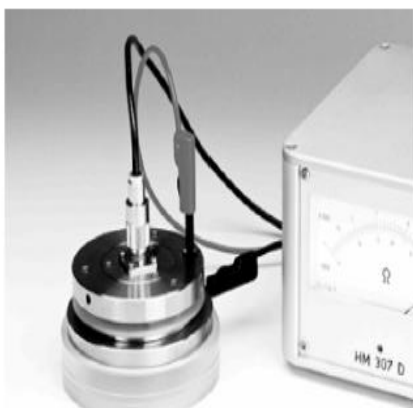
Fig. 1 Three-electrod system for measuring surface resistivity [4]
