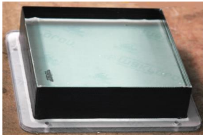
Fig. 4 Example of transparent armor for a vehicle window
