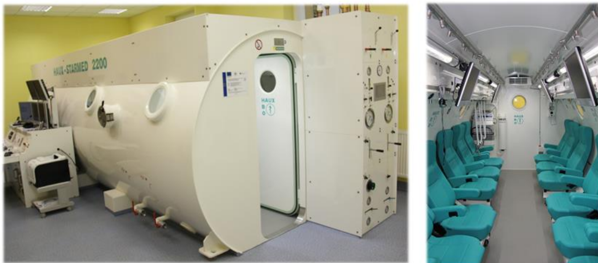
Figure 1: Multiple seat chamber of the Centre for hyperbaric oxygen therapy, Faculty of healthcare, ADU Trenčín
