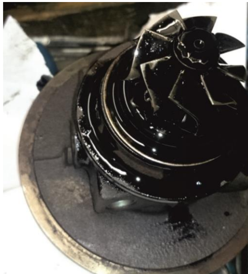
Fig. 2 Turbocharger with damaged rotary seal
