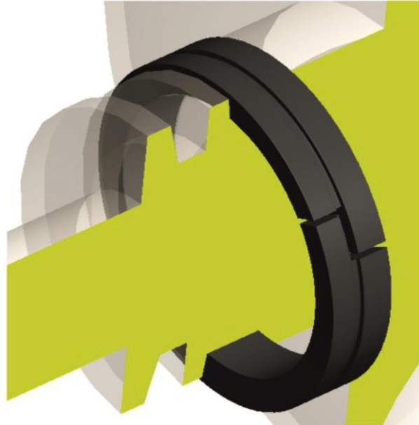
Fig. 5 Rotary seal impeller of the turbine – design
