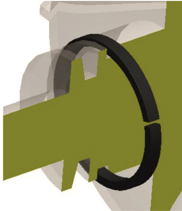
Fig. 4 Rotary seal of the impeller turbine
