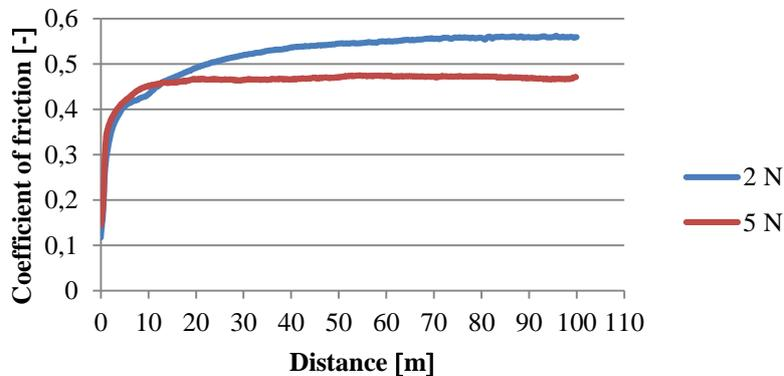
Fig. 7 The behaviour of friction coefficient on HCM 18 substrate
