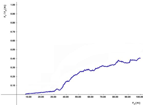
Fig. 6 The behaviour of friction coefficient
