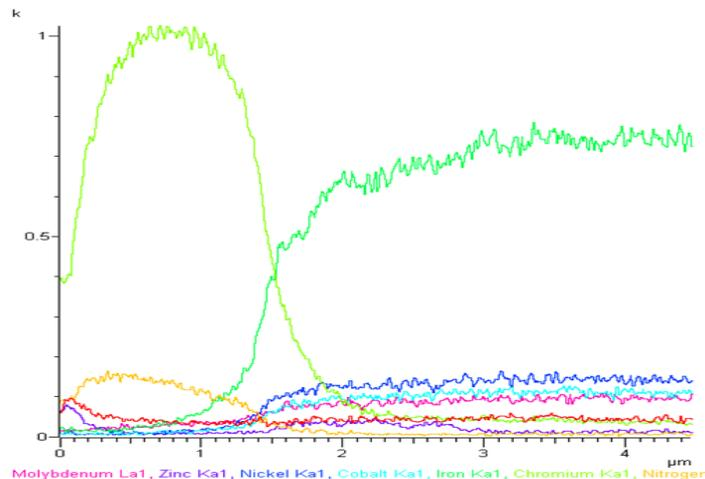
Fig. 3 Elements contained in the deposited layer CrN
