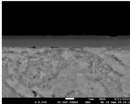
Fig. 2 Microstructure-substrate interface layer
