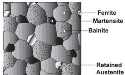
Fig. 3 Schematic microstructure of TRIP steel [3]
