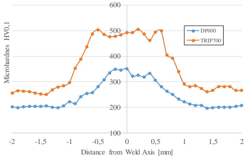
**Fig. 2** Course of microhardness across welding joint
