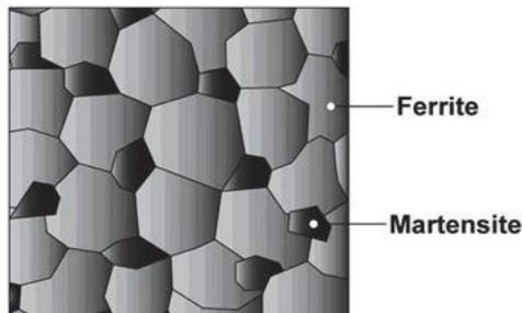
Fig. 2 Schematic microstructure of DP steel [3]
