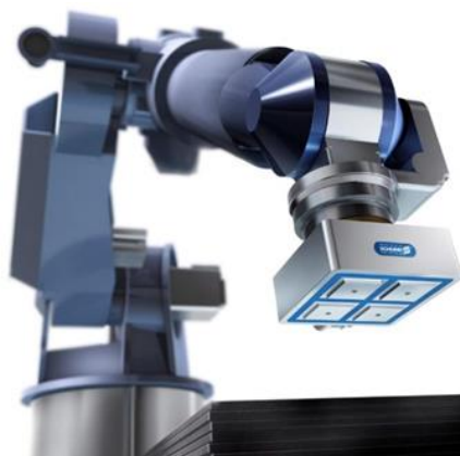
Fig. 4 Effector consists of an electromagnet [3]
