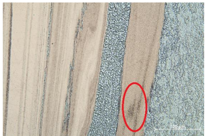
Figure 5 Microstructure of heterogeneous friction weld steel 23B2 – copper [1]
