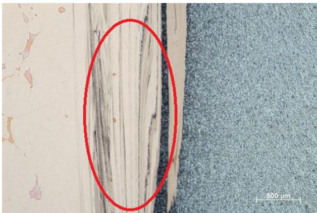
Figure 4 Microstructure of heterogeneous friction weld and the area around the weld steel 23B2 – copper [1]
