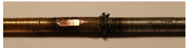
Figure 2 Heterogenous friction weld steel 23B2 - copper, specimen without modification [1]
