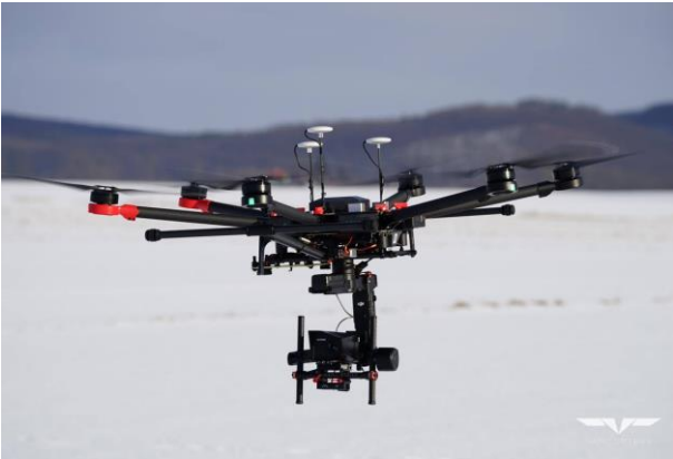
Fig. 2 UAV DJI M600 with thermo camera Workswell WIRIS
