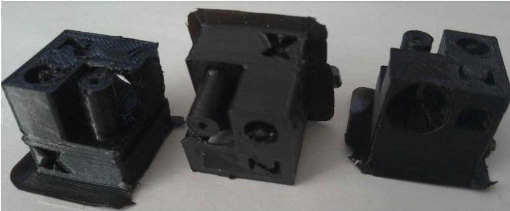
Fig. 4 Test specimens made of FLEX material
