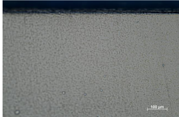
Fig. 5 Material M390 structure etched by Nital
