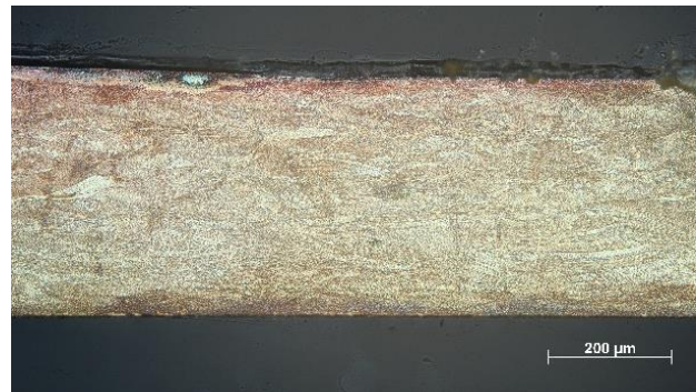
Fig. 3 Structure of CuZn30 brass after deformation
