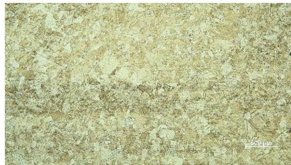
Fig. 4 Structure of CuZn30 brass after recrystallization
