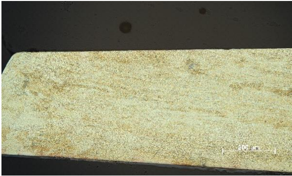
Fig. 8 Structure after first drawing
