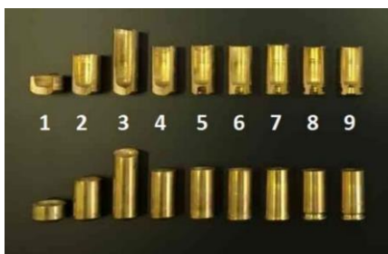
Fig. 2 9x19 Luger cartridge case manufacturing process
