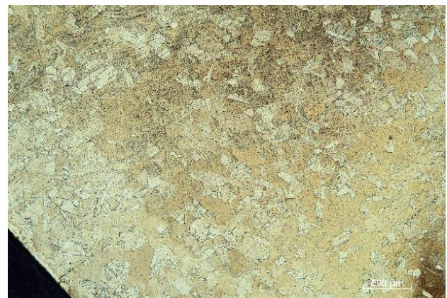
Fig. 7 Structure of entry semi-finished product cup after recrystallization
