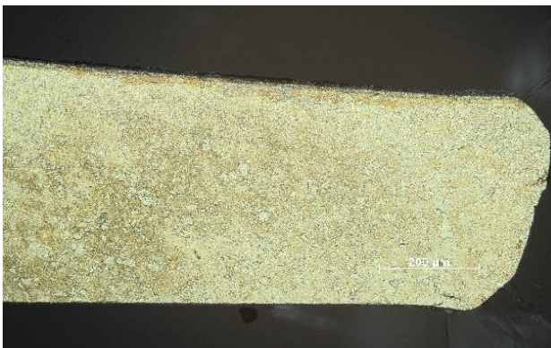
Fig. 9 Structure after first drawing and recrystallization
