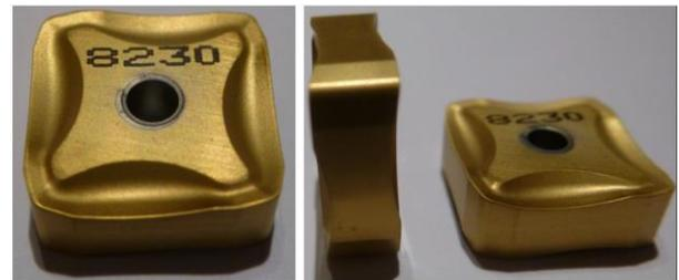
Fig. 2 Geometry of tested cutting inserts used in the face milling process
