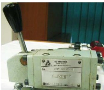
Fig. 6 Four-way and two-position switch valve 4/2 RSP1-062J15-1
