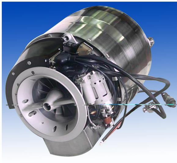
**Fig. 1** Image of turbojet engine TJ 100
