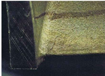
Fig.5 The turbine wheel with the crack of blade
