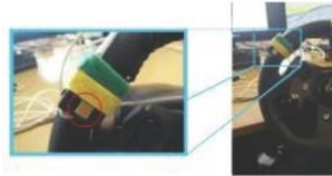
Fig. 5 The set-up of the thermal steering wheel. The Peltier element can be seen on the left (red circle) mounted on a heat sink.
