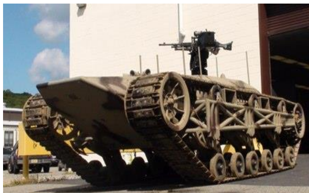
Fig. 7 Remote controlled unmanned vehicle Ripsaw, [15]
