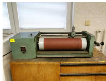
Fig. 5 Device for a rapid wear testing
