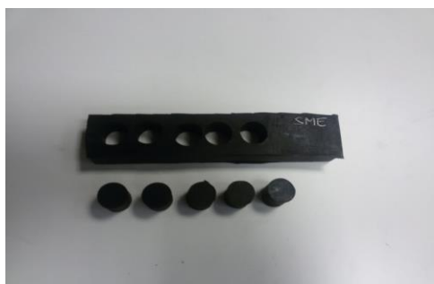
Fig. 4 The samples for a rapid wear test
