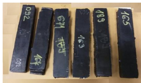
Fig. 2 The bodies for the preparation of samples for quick wear testing
